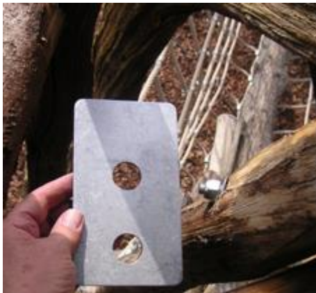
Entrapments in a downwards direction
