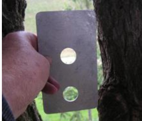
Entrapment in a sideways direction
