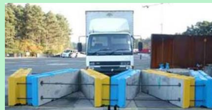
Additional wire rope added to the barrier (left and right); and the configuration changed to a 'zig-zag' shape (right).
