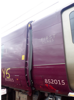
Figure 8: Damage at vehicle ends.
