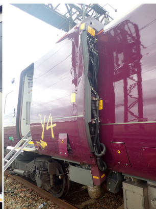
Figure 8: Damage at vehicle ends.
